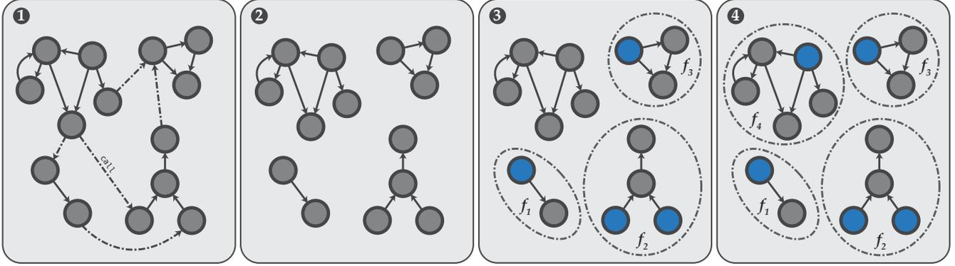
Figure 1: Overview of our function detection algorithm. ① Disassemble binary and generate ICFG. ② Hide edges  $e \in E_{call}$ . ③ Locate directly called entry points (shaded blue) and expand functions by following control flow (ignoring direction). ④ Find remaining functions through connected components analysis and detect entry points through intraprocedural control flow analysis.
